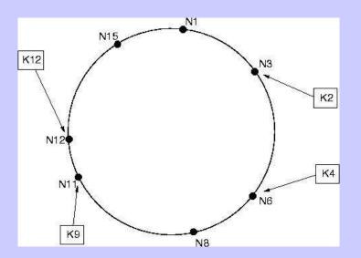
Key k is assigned to the first node whose identifier is equal or follows the identifier of k. This node is called the *successor*
